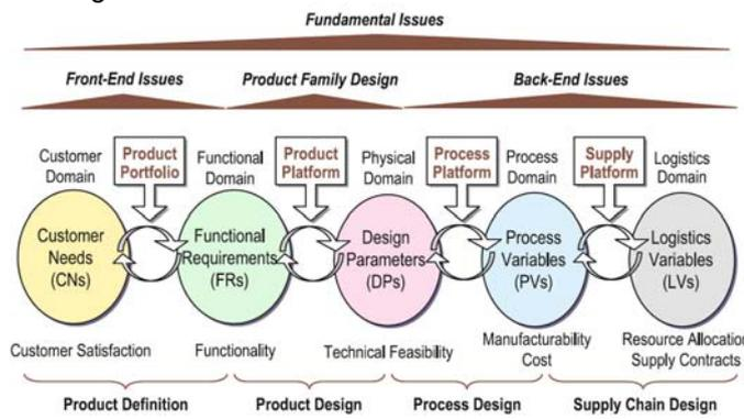
**Figure 3:** Holistic design framework covering the value chain [19]
